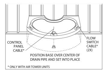
NOTE: If there is any gap between base flange and stud or blocking, shims MUST be used to prevent distortion or cracking of the flange. See Shim Instructions.
